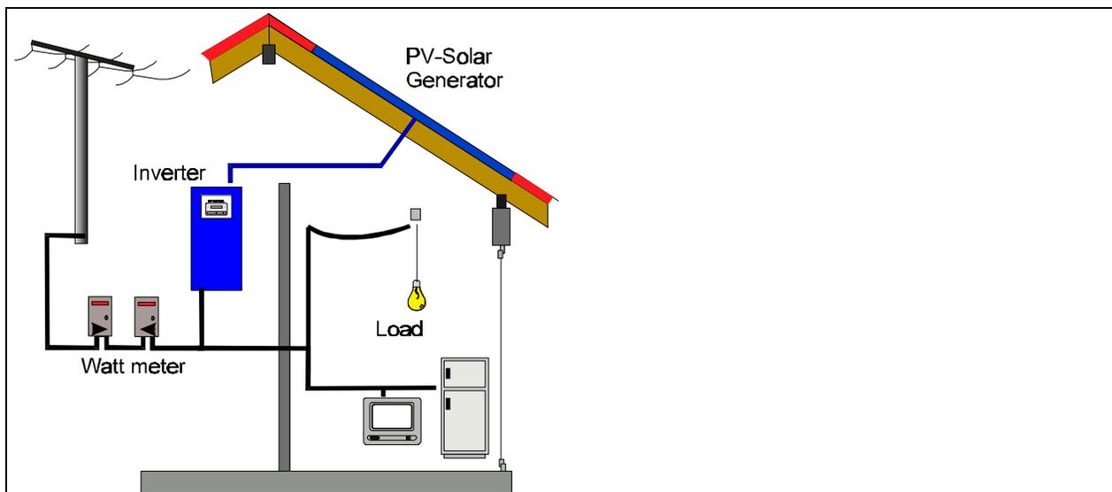
Figure 3-10 Grid Connected PV-generator for a Household
