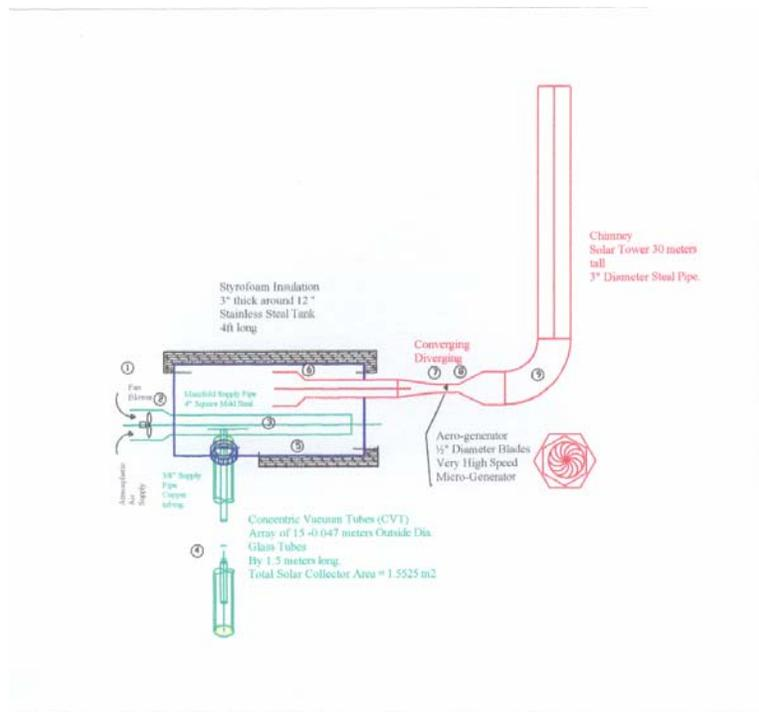
Figure #1. Schematic of proposed solar power generator.
