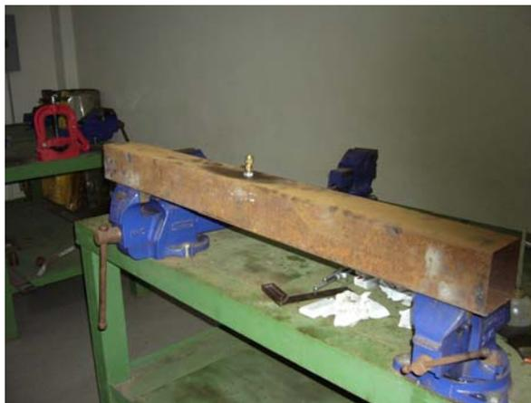
Photograph #3. Construction phase of the 4" mild steel square manifold. As can be seen a copper tubing fitting is installed to support supply pipe inside vacuum tubes.
