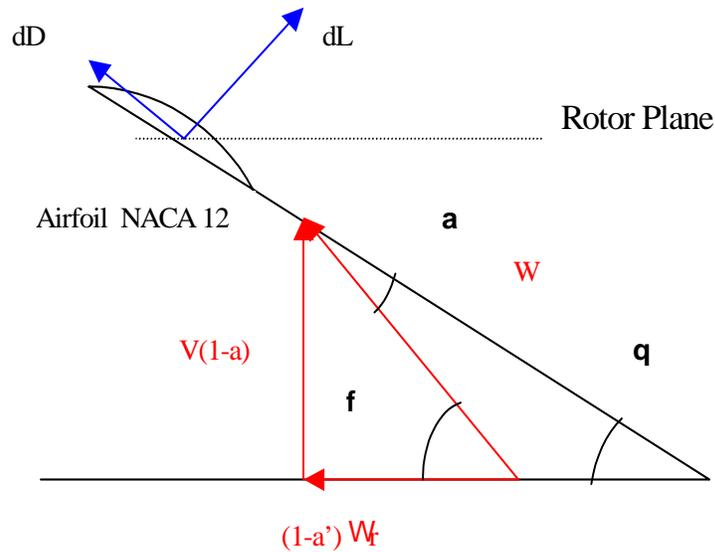
Figure #2. Velocity and Forces acting on a blade of aero-generator.
