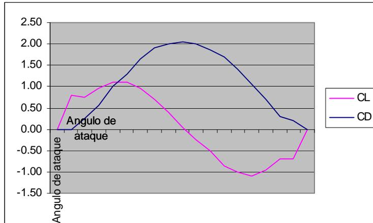
Figure # 3. Airfoil correlations for NACA 0012, Lift and Drag coefficients.<sup>⊕</sup>
