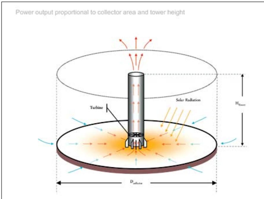
Fig. 2: Principle of the solar updraft tower (Schlaich Bergermann Solar, Stuttgart).
