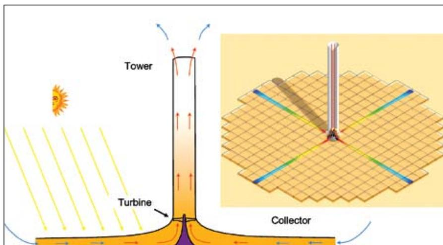
Fig. 1: The solar updraft tower built at Manzanares, Spain, in 1982 (Schlaich Bergermann Solar, Stuttgart).
