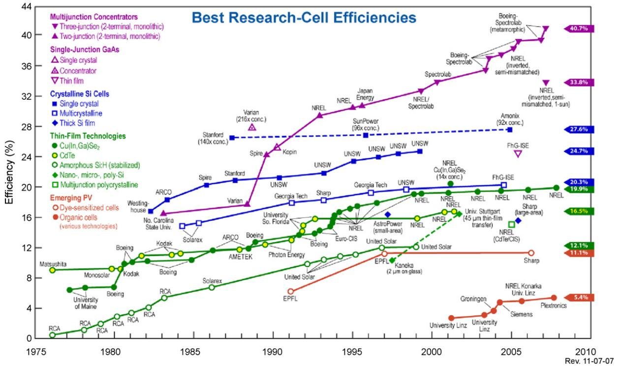
Fig. 1. Temporal development of best PV cell efficiencies, Courtesy of L.L. Kazmerski, National Renewable Energy Laboratory (NREL).
