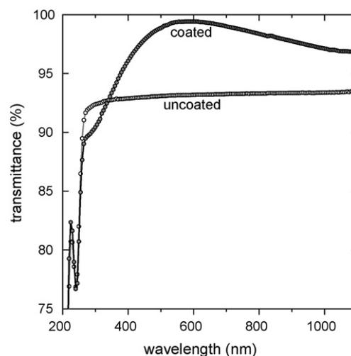
Fig. 3. Spectral transmittance of a cover glass for a high-temperature cavity receiver of solar tower plants: silica glass (4 mm) and coated with porous SiO<sub>2</sub>-bearing sol-gel layer.
