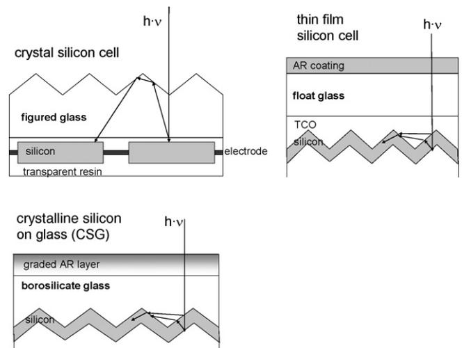
Fig. 2. Coated and figured solar glasses as part of crystalline silicon, thin-film silicon and crystalline silicon on glass cell concepts. Arrows indicate paths of multiple reflections.
