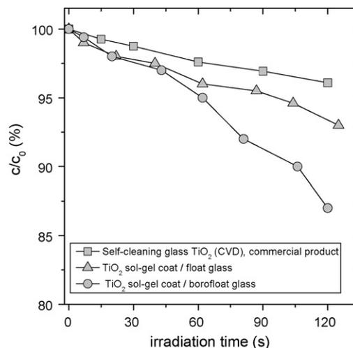
Fig. 4. Degradation of dichloroacetic acid ( $c_0 = 5 \text{ mmol l}^{-1}$ ) as a function of UV-A irradiation time (thin-film reactor,  $60 \text{ W m}^{-2}$  UV-A) of  $0.024 \text{ m}^2$  sized samples of commercial self-cleaning glass ( $\text{TiO}_2$ -CVD coat), soda-lime-silica float glass ( $\text{TiO}_2$  sol–gel coat), and borofloat glass ( $\text{TiO}_2$  sol–gel coat).
